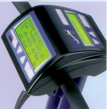
Programmable control unit with two displays for both the operator and the test subject
