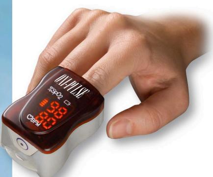
Sensor and display are combined in a pocket sized, lightweight device in which the patient directly inserts his finger.
